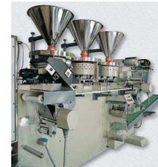
Upto four independent feeding systems can be mounted to produce multi-product packs.
